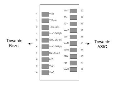
Pin-out of connector Block on Host board
